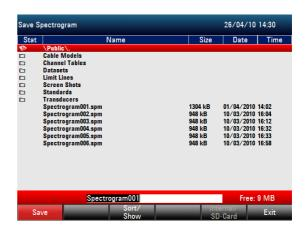
The number of spectrograms that you can store on the R&S FSH's internal memory depends on the other datasets that are currently on the R&S FSH.
