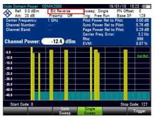
The y-axis represents the power of the signal. The power of the codes is relative either to the total power of the signal or relative to the power of the pilot channel (PICH).
