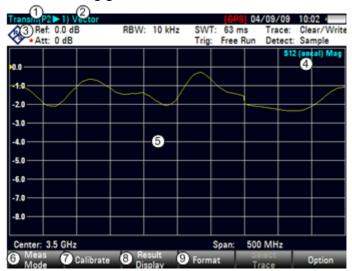
When the tracking generator is switched on, the status line indicates (Uncal). This indicates that tracking generator measurements are uncalibrated. The level axis is in the relative unit dB. Apart from the level values, the 0 dB reference is also displayed. This corresponds to a reference level of 0 dBm in the spectrum analyzer mode (= nominal output level of the tracking generator).
