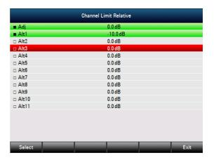
To deactivate the limit check for a specific channel, move the cursor to the channel in question with the rotary knob or the cursor keys and deselect it with the SELECT softkey.
