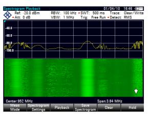
Therefore you should adjust the color map to the overall shape of the signal you are measuring. Let's say, for example, that the signal has an amplitude range of about 30 dB with the maximum amplitude at about -60 dBm and the minimum amplitude at about -100 dBm and the Green-Yellow color scheme. With the default settings, the spectrogram is made up exclusively of green colors and it's not easy to distinguish amplitude levels. That's because the yellow color shades are completely out of range.
