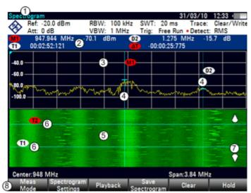
By default, the spectrogram result display consists of two windows. The upper window shows the measured spectrum as a trace line. The lower window shows the measurement results in a spectrogram. The chronological information in the spectrogram is restricted by the internal memory of the R&S FSH. The R&S FSH stores 1024 frames or spectrums that have been measured in its memory. As the height of the display is smaller, some of the data becomes invisible after a time.
