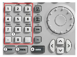
If the R&S FSH is expecting a letter entry, it automatically assigns the letters above the keys to the keys in the alphanumeric keypad. The keys have a multiple assignment. Enter the letter you want by pressing the key in question the appropriate number of times.
